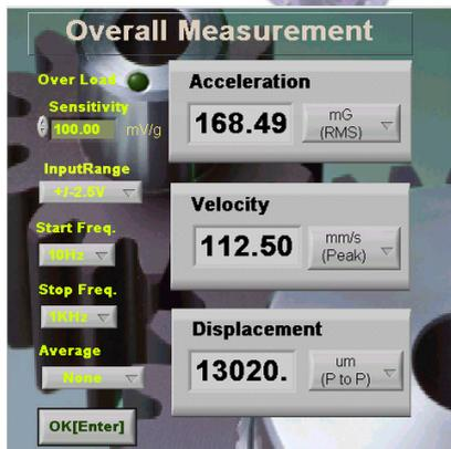
Vibration meter mode enables you to measure vibration levels of acceleration, velocity or displacement.
