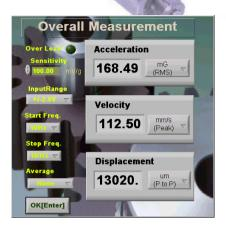
Vibration meter mode enables you to measure vibration levels of acceleration, velocity or displacement.
