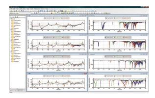
Signal map for FFT analysis: Map functions: time waveform, auto power spectrum, complex spectrum and cross spectrum; Measurement controls: free run, armed by time step or armed by rpm step; Display signal map in waterfall plot or intensity map.
